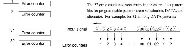
This bit window can be combined with the block window (4.4.7) to measure a 1 bit error in the measurement pattern.
