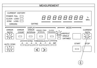
When you want to display the result during measurement, press the CURRENT DATA key. The LED inside the key lights. When CURRENT DATA is ON, the current measured result is displayed at eachmeasurement time. (See 4.5.11.)
