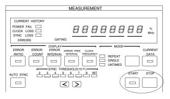
When the START key is pressed, the start lamp lights and measurement starts in accordance with the measurement mode.
