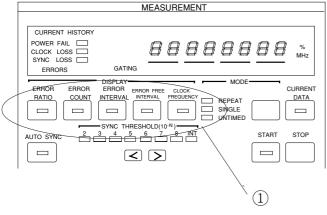
① Select the item to be displayed at DISPLAY from among error ratio, error count, error intervals, error free intervals, and clock frequency.
