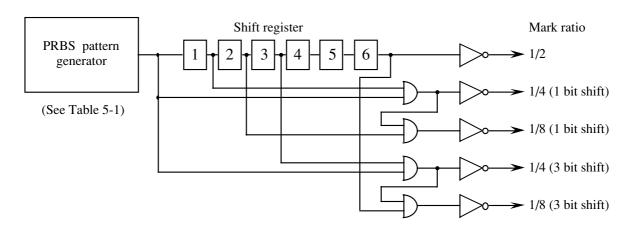
Fig. 5-1 Mark Ratio 1/4, 1/8 Pattern Generation Circuit
