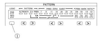
Each time the LOGIC key is pressed, the logic of the set pattern changes in positive → negative → positive order. (The set logic is shown by lighting of the lamps.)
