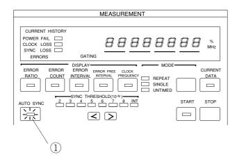
① In normal measurement, the AUTO SYNC function is turned on and input pattern and comparison pattern synchronization is established automatically. To turn on the AUTO SYNC function, press the AUTO SYNC key. The lamp inside the key lights.
