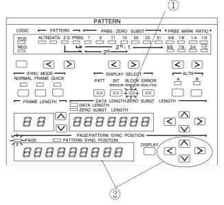
① Press the BLOCK WINDOW key of DISPLAY SELECT to light the LED inside the key.
