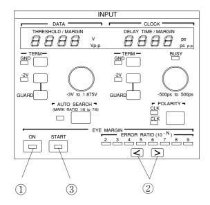
① Press the ON key. The LED inside the key lights. At this time,
