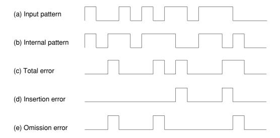
Fig. 4-4 Error Detection Mode
