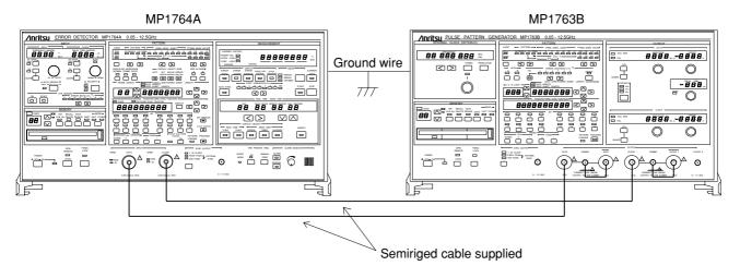
Fig. 7-1 MP1763B and MP1764A Setup
