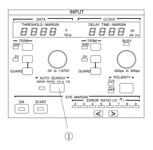
① When the AUTO SEARCH key is pressed, the DATA threshold voltage and CLOCK Delay are automatically set. If AUTO SEARCH does not end within three seconds, AUTO SEARCH stops and the AUTO SEARCH lamp begins to blink. At this time, return the data threshold voltage and CLOCK delay time to the set value before AUTO SEARCH.
