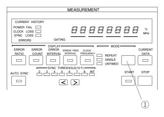
Press the MODE key and select the measurement mode.
