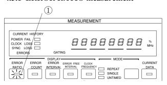
① Press the ERROR RATIO key. The LED inside the key lights and the ERROR RATIO measured result is displayed at DISPLAY.
