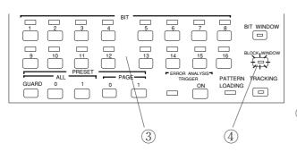
One LED of the BIT indicator indicates one bit in the pattern setting. When one key of the BIT indicator is pressed, the LEDs for all 32 bits go on or off together because the block window is turned on or off for each of the 32 bits.
