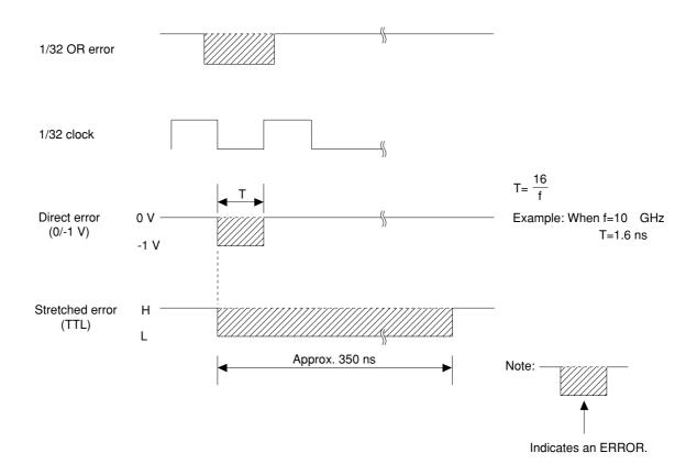
Fig. 5-5 Error Output Pulse
