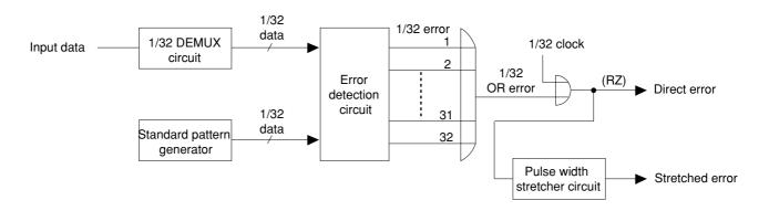
Fig. 5-4 Error Output Block Diagram
